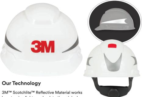
3M™ Scotchlite™ Reflective Material works by returning light rays back to the original source, a result of the retroreflective properties of thousands of microscopic glass beads incorporated into the material.
