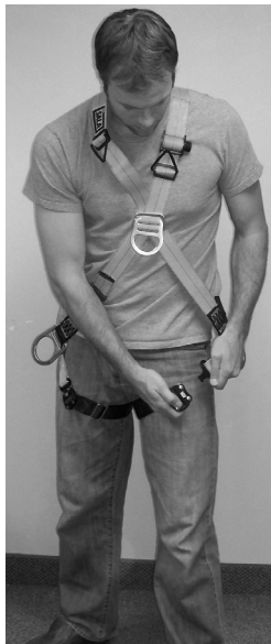
Figure 12 - Installing the Belt (Crossover-Style)
